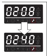
The multifunctional display pane will present a prompt similar to the example shown at left, with the first digit of the four-digit configuration code flashing.
